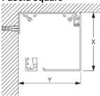
Fascias can be top or face fixed. Ensure you have a flat fitting surface which will accommodate the depth of the top profile.
