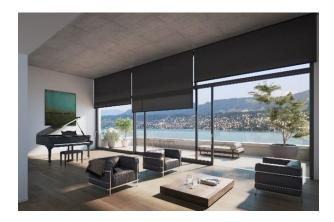
Fascias and headboxes conceal the roller blind barrel, creating a sleek and polished look. They blend seamlessly with the window reveal, or even disappear into the ceiling, giving the illusion that the fabric is cascading directly from above.
